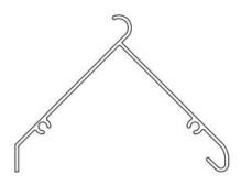
MINIMUM PITCH - 45mm (24mm COVERAGE) NOMINAL PITCH - 61mm (8mm COVERAGE) MAXIMUM PITCH - 67mm (2mm COVERAGE)
